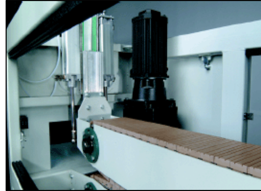
Guidance and drive of caterpillar
