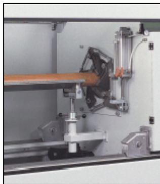
Pipe guiding during cutting
